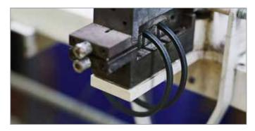
Splicing is used when an application requires a continuous seal such as a multi-sided frame or an o-ring.
